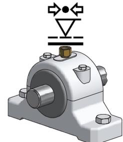
Pressure check: Lube-point / all connecting parts
