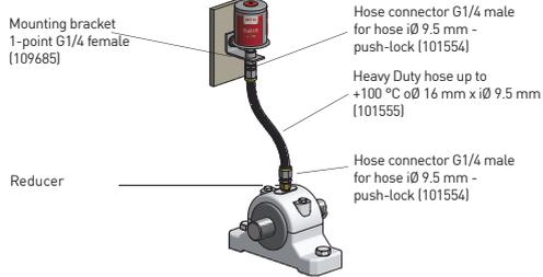
Remote mounting → for lube-points with vibration, limited mounting space, high temperature
