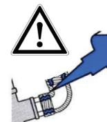
4. Lubrication point, accessory parts and tubes must be pre-filled with lubricant. This enables the lubricant to immediately reach the lubrication point.
